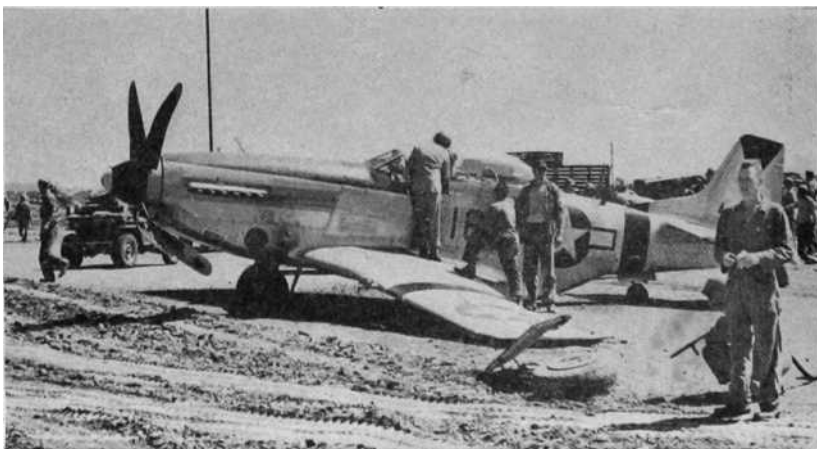
PILOT OF THIRD P-51 to land on Iwo Jima climbs hurriedly from the wrecked plane (above), after shrapnel on runway punctured tire, as crew chief beckons aid. Mechanics (right) rushed to inspect the landing damage.
